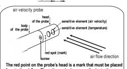
face to the airflow. Then, the probe is perpendicular to the airflow.
