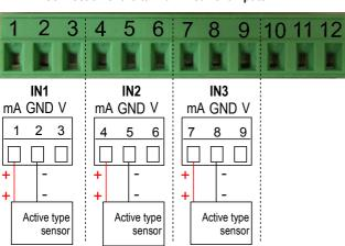
Connection of the0-5/10 V voltage inputs :
