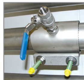
B Spot drilling collar
