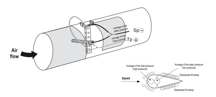
Profiled in plane wing limiting the head losses (<3%) and the turmoils.
