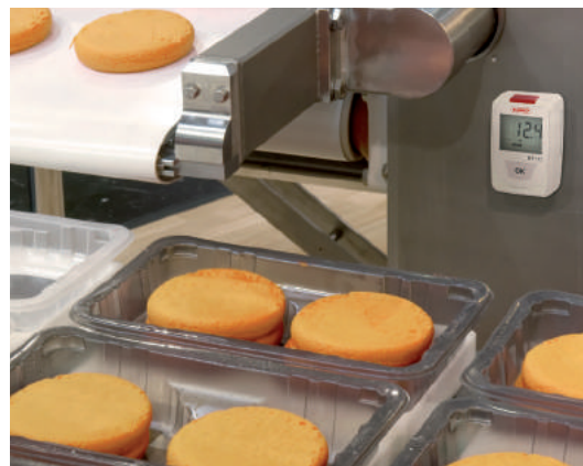
IP65 casing, compliant with the standard required by the agri-food industry
